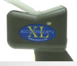
Lever the mouthpiece downward so the 2 holes on the flat side line up with the 2 inlet ports.
