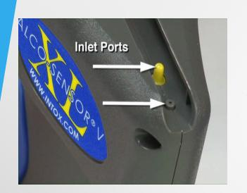
Notice there are 2 inlet ports in the channel. The smaller inlet is for the flow sensor which monitors the breath flow.
